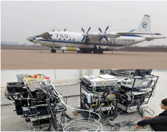
Fig. 2. Photographs of the IPDA lidar system onboard Yun-8 aircraft.
